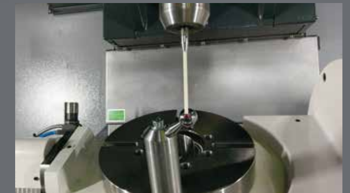
Tool Setting Probe is Standard Accessory (BLUM Model Z-nano shown)
