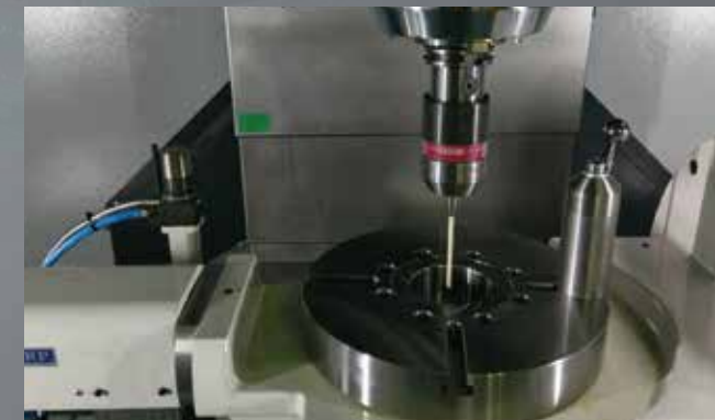
Work Piece Probe is Standard Accessory (BLUM Model T-60 shown)
