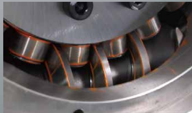
Roller Cam Bearing components used in Trunnion Table
